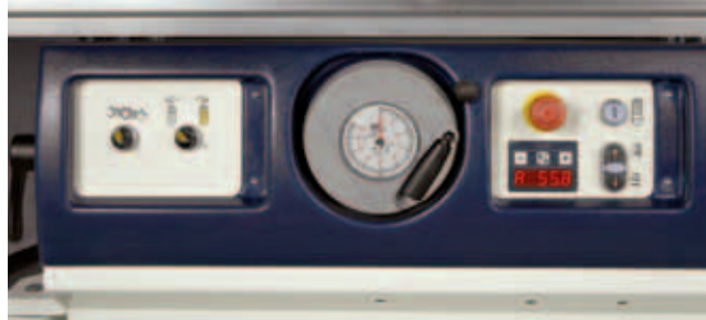
Easy to use Powered vertical movement of all operating units (spindle moulder and thickening planer with digital readout)
