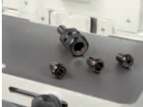
5-10-16 mm chuck with clamp.
