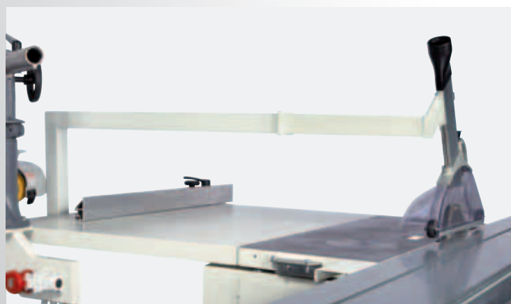
Overhead saw guard N.B. Available only on ST5 N.B. Standard for C.E. and USA/CANADA versions
